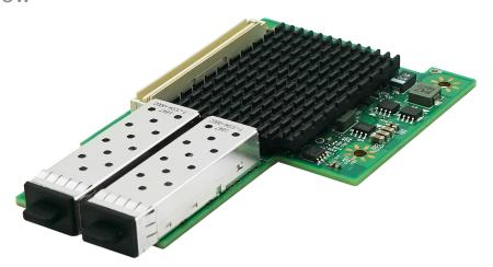
LRES3001PF-OCP is OCP Type-1 10 Gigabit dual port fiber optic Ethernet server adapter card independently developed by Shenzhen Lianrui Electronics Co., Ltd. based on the online chip control scheme of Netswift SP1000A. The card is designed for server-oriented and high-end devices. This server adapter makes it easy to share the more efficient servers and data centers in the general IT industry.
